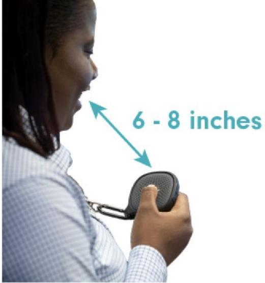
For best results, do not hold the Relay device right up to your mouth to communicate.
