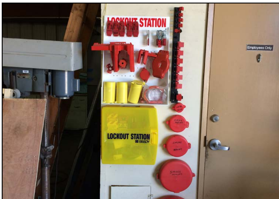
SMHS – Lockout / Tagout Center Installed in the Maintenance Shop
