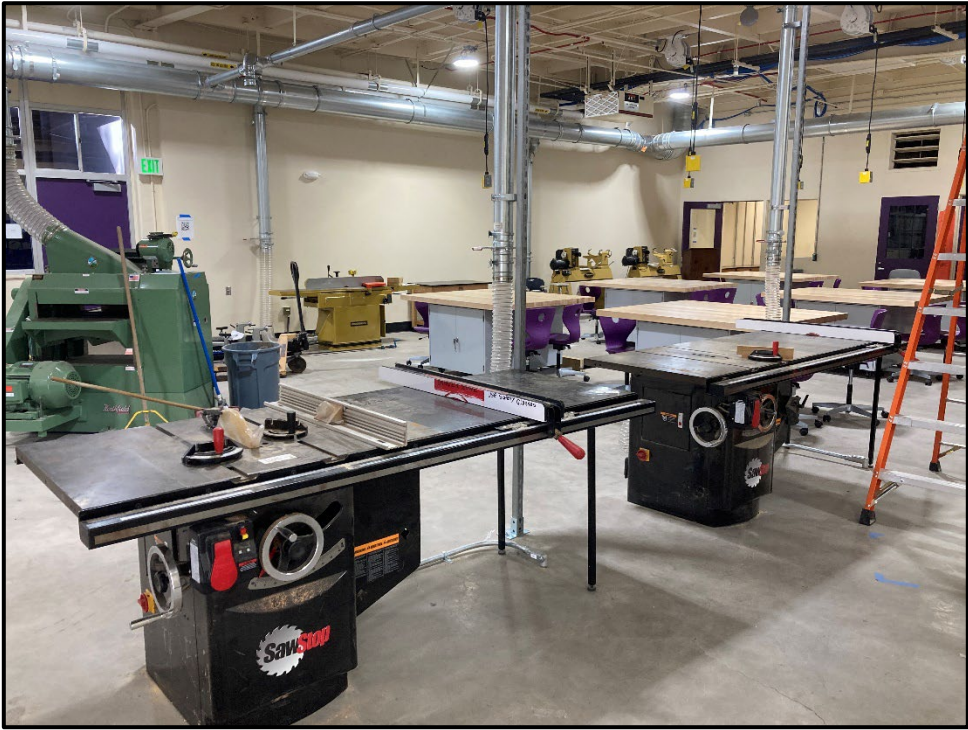
ERHS CTE Modernization – New Table Saws are Installed in the Woodshop Classroom
