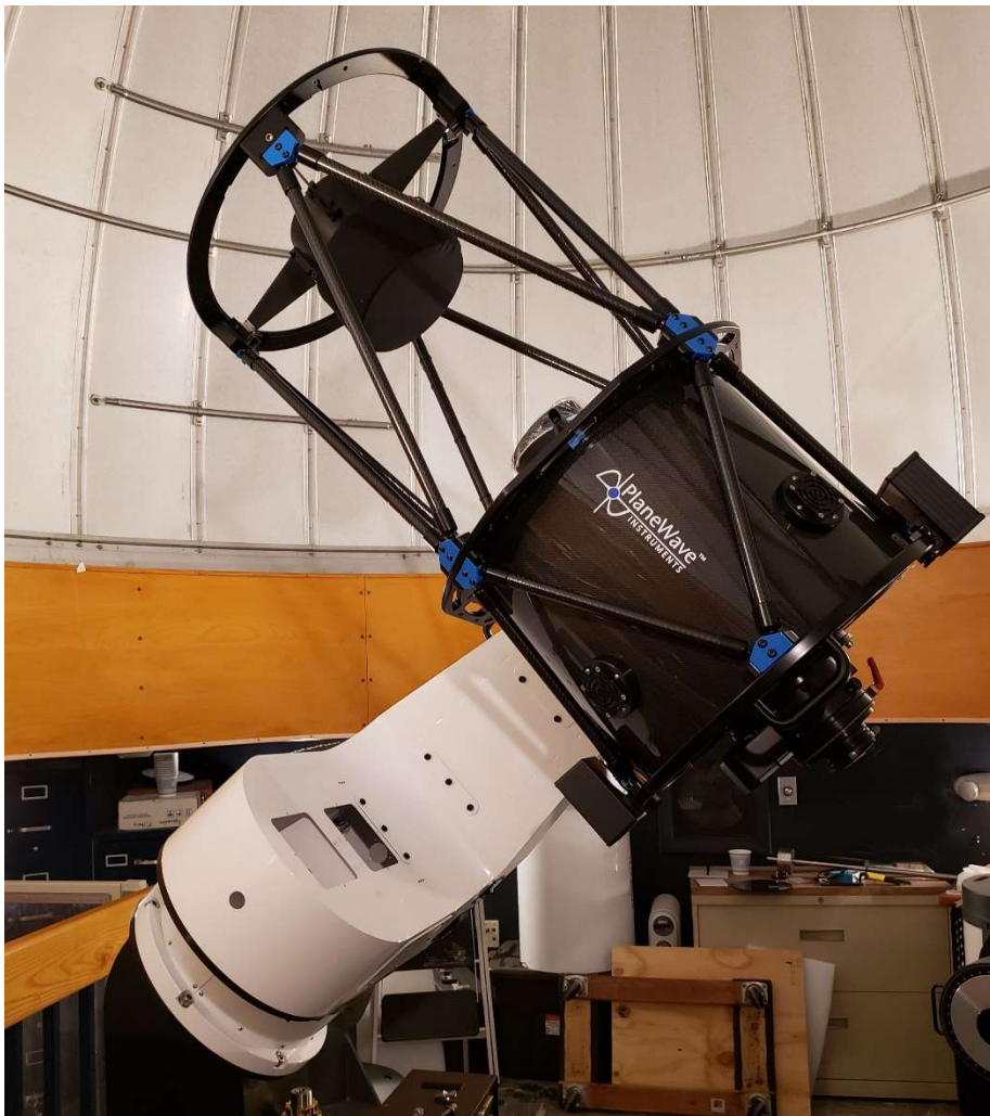
Photo: A PlaneWave CDK400 Observatory system consisting of a 17" Corrected Dall-Kirkham telescope and an L-500 direct drive mount installed at JJMO. Installation was completed on April 22, 2024.
