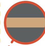
**Galvanized Pipe:** Lead particles can attach to the surface of galvanized pipes. Over time, the particles can enter your drinking water, causing elevated lead levels.
