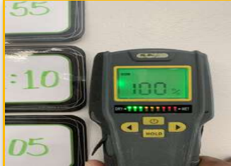
Location: ROOM 3 1.3 100% Moisture Detected/Wall
