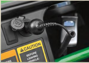
12-volt DC outlets The same kind you'll find on most Gator™ UV's are similar to the ones in boats and trucks. Keep your phone charging at all times.
