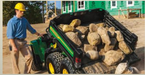
A standard gas assist shock underneath the bed makes lifting and dumping effortless. An optional power lift kit raises and lowers bed from a switch right on the dash.
