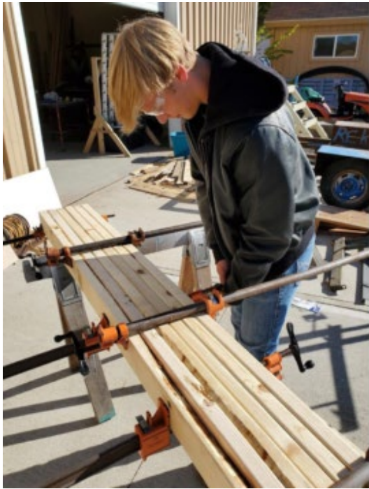
(Left) Zach Egeland gets the process underway by gluing and clamping 12-foot 2x4's together. (Right) A team of students plane the sections of glued wood.
