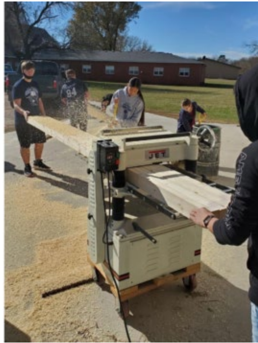
(Left) Zach Egeland gets the process underway by gluing and clamping 12-foot 2x4's together. (Right) A team of students plane the sections of glued wood.
