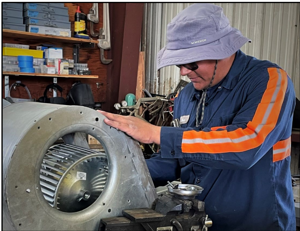
SMHS – Alex Anguiano-Alcaraz Replacing an Air Conditioning Blower Motor
