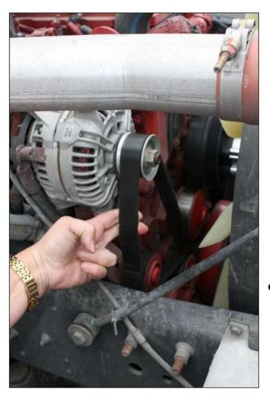
With the engine off, point to, touch, or press the belt to see that it is snug. You must push the belt with your hand. If it deflects more than 1/2 to 3/4 of an inch, you will observe that slippage is probably excessive.
