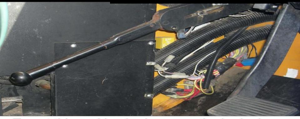
To set this parking brake move the brake lever down until it clicks into place. To turn off the parking brake push the button that releases the lever and move the lever to its proper position. It is different depending on your bus
