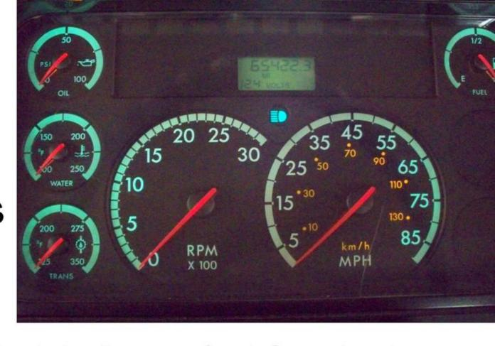
Check that dash indicators for left and right turn signal, 4-way flashers, and high beam illuminates when corresponding lights are turned on.
