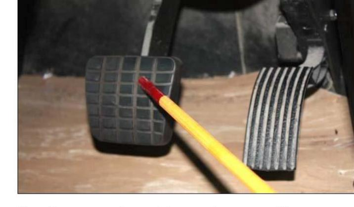
Driver pulls forward at 5 mph, applies service brake to check that brakes are working properly and to see if the vehicle pulls to one side or the other.
