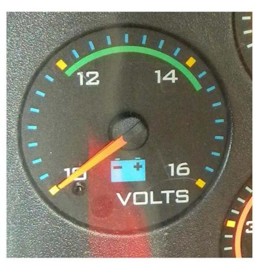
With key on and the engine running, ensure the Volt Meter gauge is operational and charging normally. If not in proper operating range it needs to be checked.
