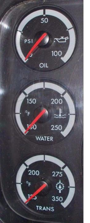
Oil Pressure Gauge With the key on and the engine running, check that oil pressure is building to normal. The gauge shows increasing or "normal" oil pressure or the warning light goes off.
