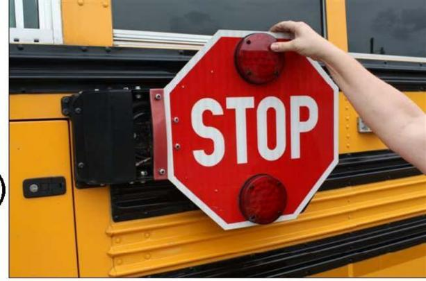
Check that signs and arm extend fully when operated.
