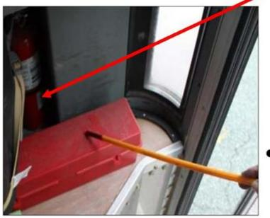
Check for a properly charged and properly rated fire extinguisher. Make sure it is secured properly.
