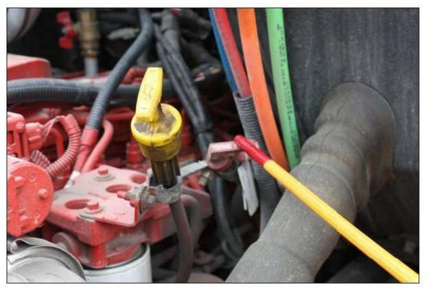
Driver should mention that you check the transmission level while the engine is running. The engine should be hot and at the transmission fluid is at the proper level.
