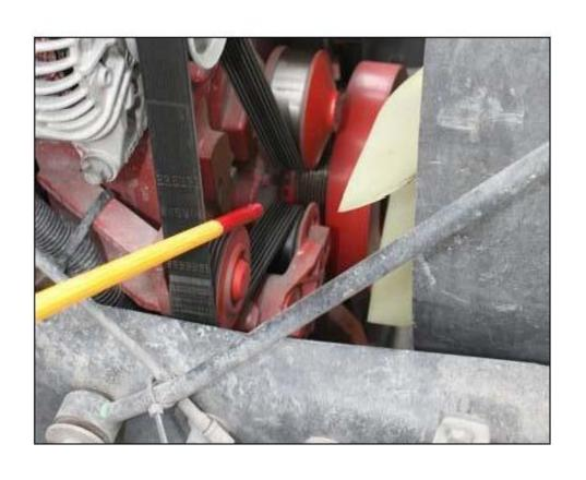
Correctly identify the water pump. Check that the water pump is mounted securely. Check that the water pump isn't leaking. Identify that water pump is belt driven.
