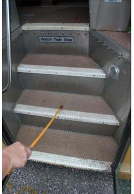
Check that entry steps are clear with the treads not loose or worn excessively.
