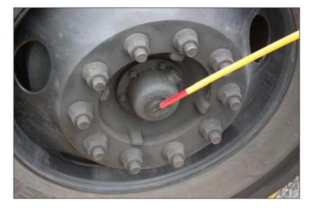
Check that hub oil seal is not leaking and has adequate fluid.
