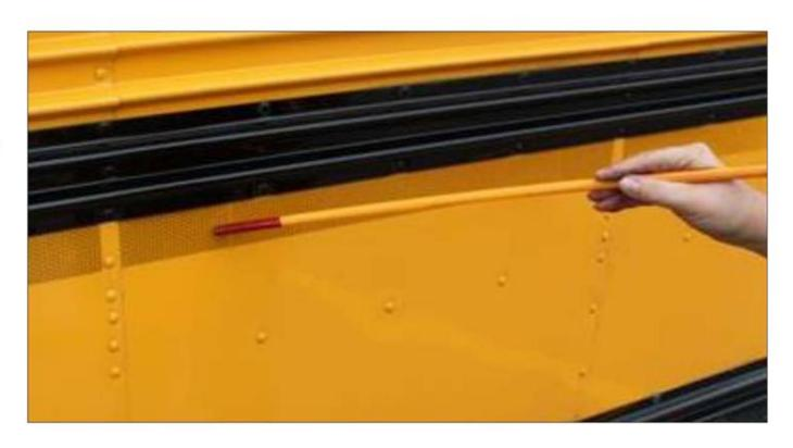
Check that reflector tape is clean, none of the tape is missing or cracked, and they are the proper color.
