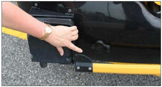
Check the stop arm to see that it is mounted securely to the vehicle and it is not damaged.
