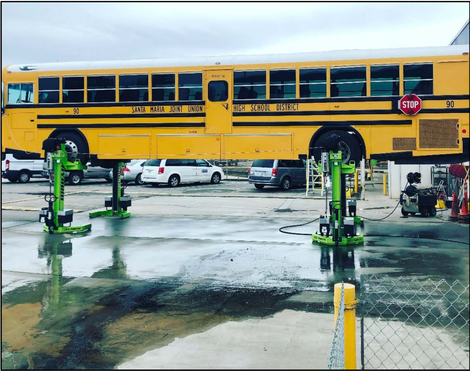
Transportation - Mobile Bus Lift Used to Steam Clean Undercarriage
