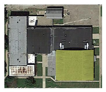
The existing roofing will be removed down to the wood substrate. A synthetic underlayment will be installed on top of the substrate, and new asphalt shingles will be installed.
