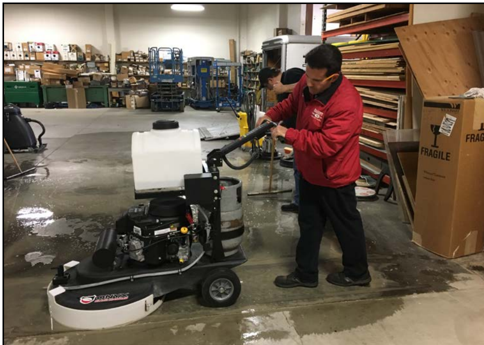
SMHS – Ken Groppetti Tests a Concrete Polisher
