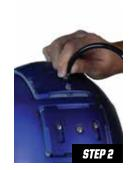
Lubricate the pump needle generously and insert needle as shown. Do not force the needle into the port; doing so may puncture the liner's opposite wall.
