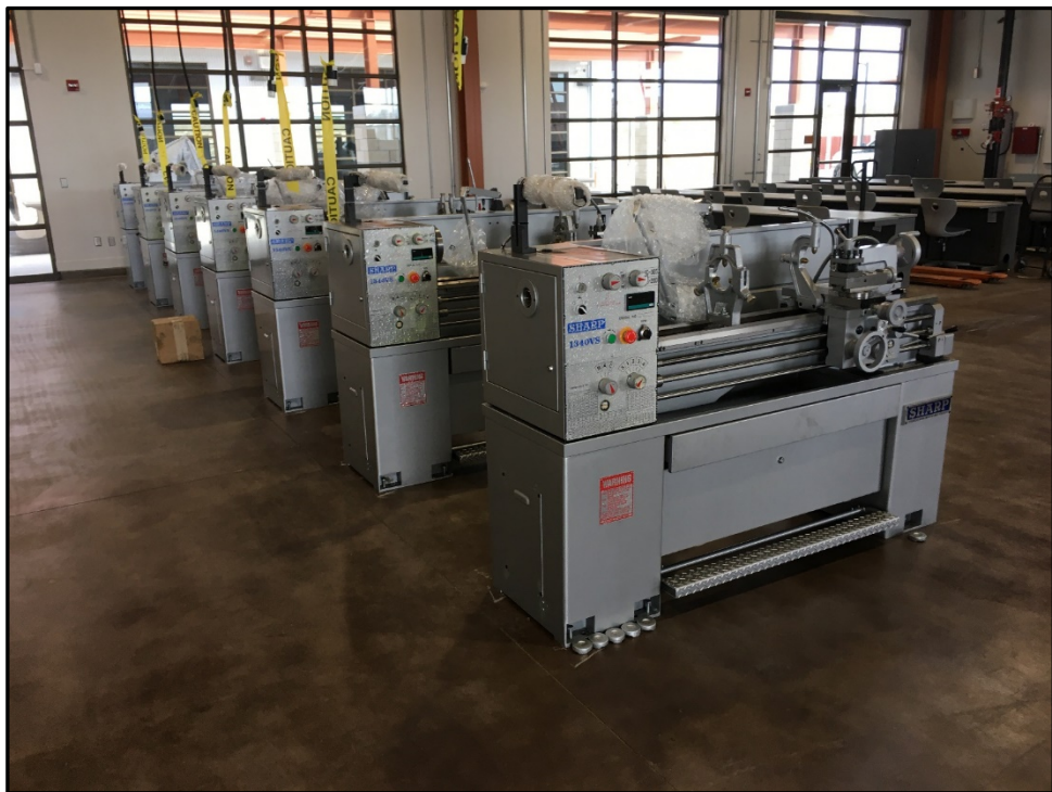
CTE Center – Seven Engine Lathes all in a Row
